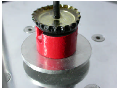
Figure 2 Magnetic location of sample in crown cap
